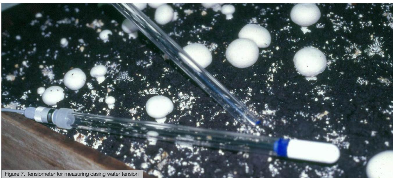
Figure 7. Tensiometer for measuring casing water tension
